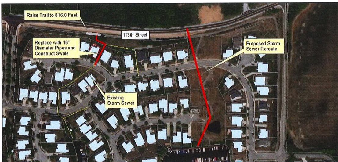
Figure 10 – Storm Sewer Reroute
